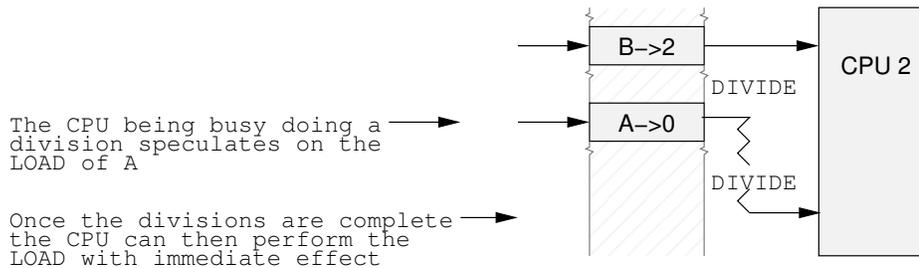
Figure 14.16: Speculative Load
