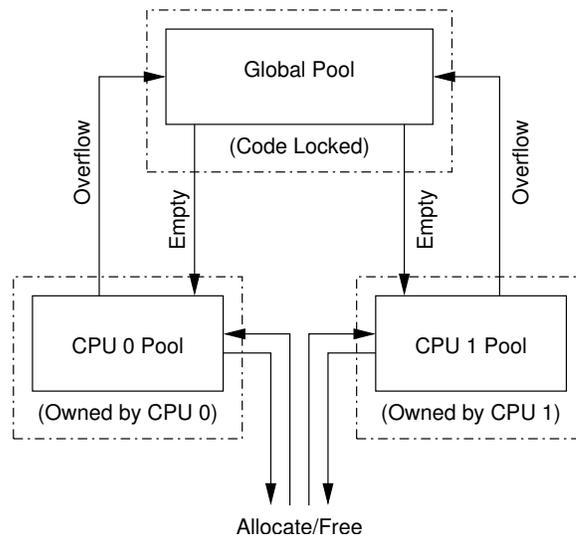
Figure 6.27: Allocator Cache Schematic
