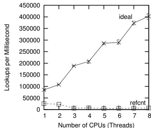
Figure 9.5: Pre-BSD Routing Table Protected by Reference Counting
