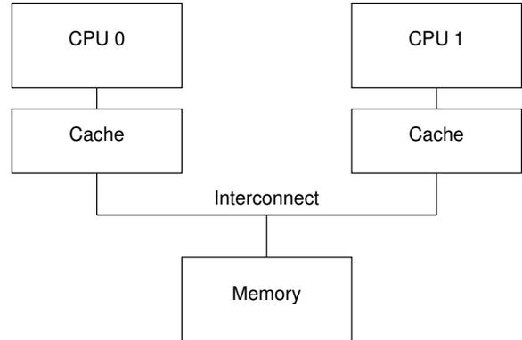
Figure 14.1: Modern Computer System Cache Structure
