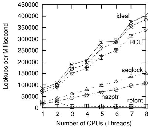
Figure 9.33: Pre-BSD Routing Table Protected by RCU QSBR
