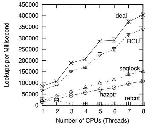
Figure 9.32: Pre-BSD Routing Table Protected by RCU
