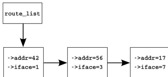
Figure 9.1: Pre-BSD Packet Routing List
