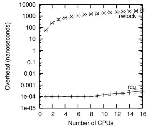
Figure 9.34: Performance Advantage of RCU Over Reader-Writer Locking
