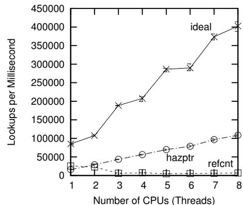
Figure 9.9: Pre-BSD Routing Table Protected by Hazard Pointers
