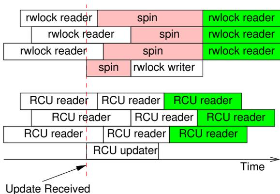
Figure 9.37: Response Time of RCU vs. Reader-Writer Locking
