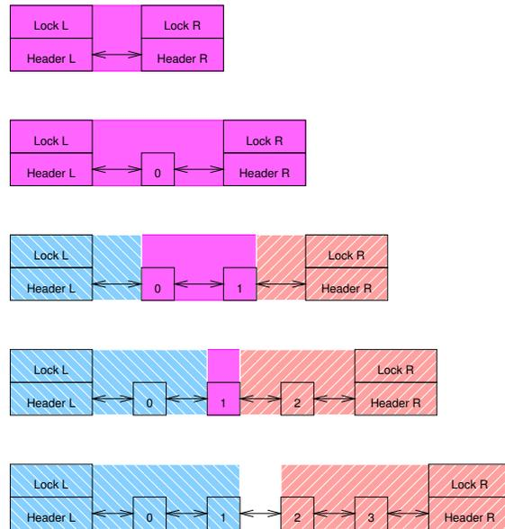
Figure 6.5: Double-Ended Queue With Left- and Right-Hand Locks
