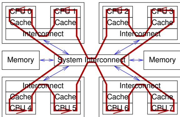
Figure 5.4: Data Flow For Global Atomic Increment
