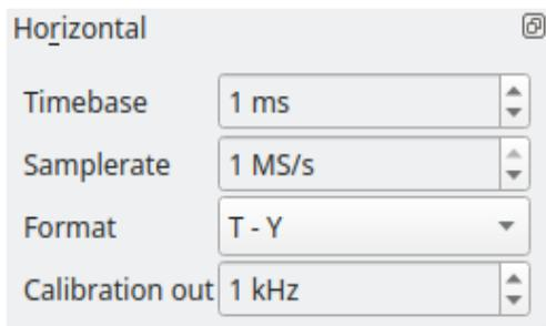
The displayed time range of the trace can be selected by **Timebase** between 10 ns/div and 100 ms/div in 1/2/5 steps. The display's width is 10 div, marked with vertical dotted lines on the screen.
