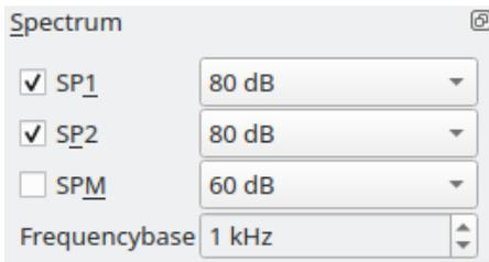
The program calculates the voltage spectrum of the three channels using the discrete FFT and displays the results if enabled.
