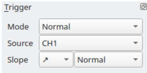
Triggering allows to display a stationary trace by fixing a rising or falling **Slope** of the signal of the selected **Source** channel to a defined position on the screen. The triggering is done in software by searching for the trigger condition in the sampled values and skipping the necessary amount of leading samples to position the trace accordingly.
