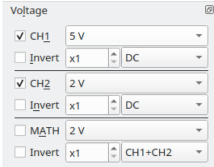
Both channels measure the voltage related to GND.
